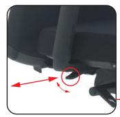
Armrest Expand Adjustment Expand adjustment procedure Push the lever down and find the required position - pull up the lever up to lock.
