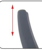
Back Height Adjustment Back height adjustment procedure Pull up the backrest upward to find the required position.
